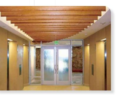
Tremolo™ [TR1] is a tapered wood baffle that furnishes a stunning and impressive appearance. Each member suspends individually by HD T-Grid. An integral light fixture can be incorporated. Tremolo™ baffles typically have a depth of  $8\frac{1}{2}$ ", and can be manufactured in a wide variety of veneer.
