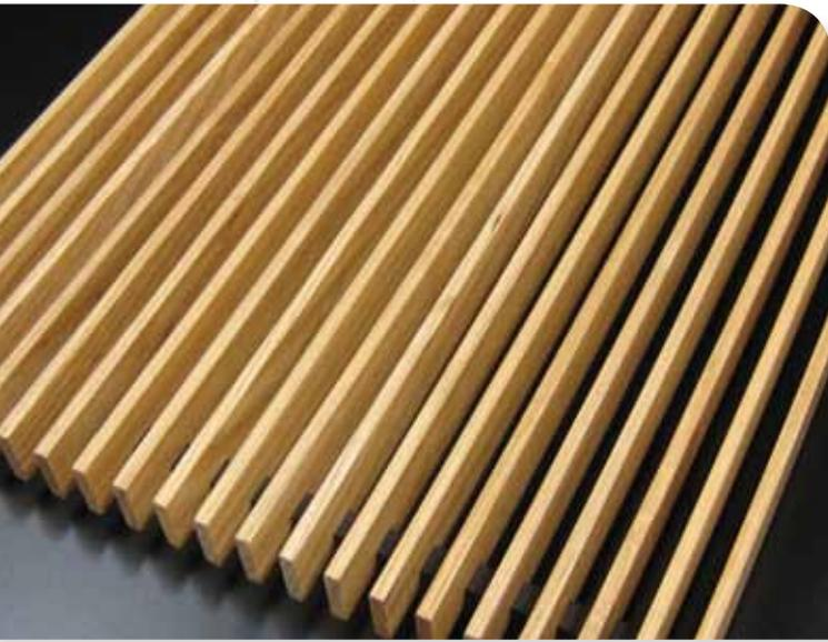
ACGI Micro-Grille series are an elegant solution for ceilings and walls. The panels offer a standard blade thickness of  $\frac{3}{16}$ " and 1" depth. Panels can extend to eight feet in length.
